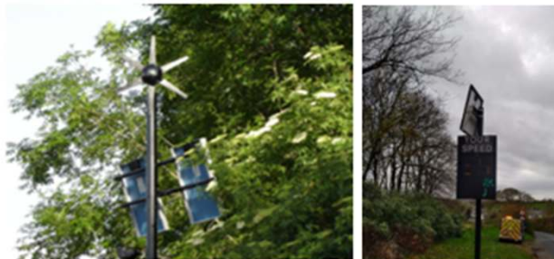
These are examples of a poor location for solar to be erected!
